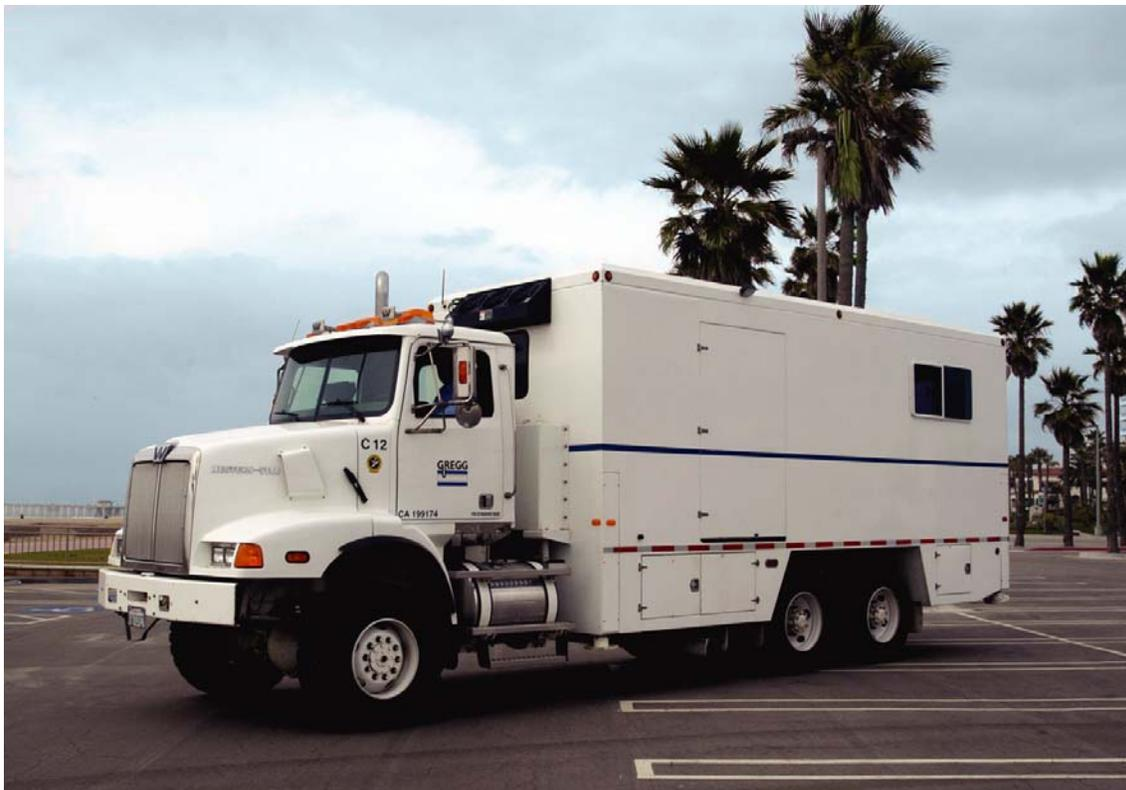
**Figure 10** Truck mounted 25 ton CPT unit
